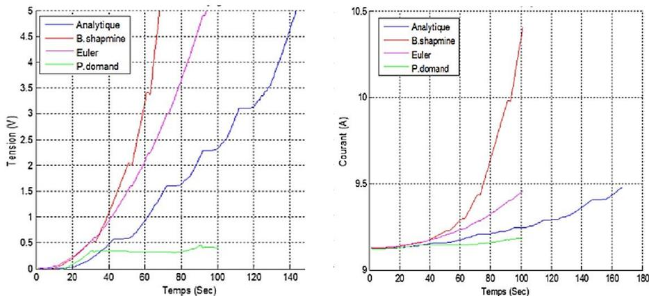
Figure.13: The characteristics of (I and V) for two BOOST in series with the evaluation of the shading effect by the different numerical methods.
