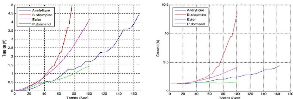
Figure.14: The characteristics of (I and V) of two BOOST in parallels with the evaluation of the shading effect by the different numerical methods.
