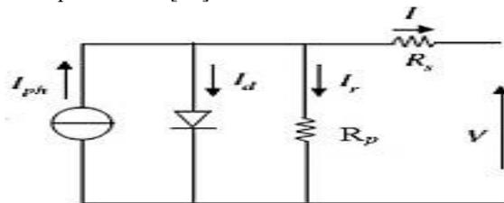
Figure. 1: General model of PV cell in a single diode model
