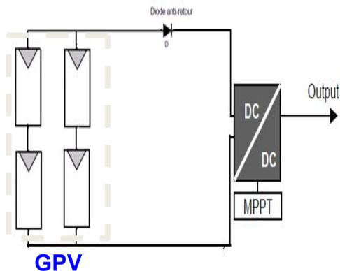
Figure.6 : Central converter configuration.
