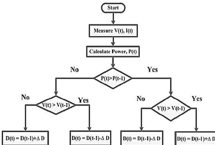
Figure. 5: Flowchart for P&O Method [6]
