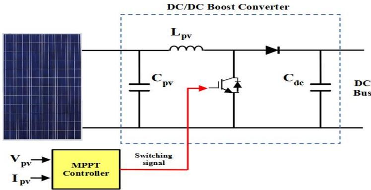
Figure. 4: Solar energy conversion system with P&O MPPT.
