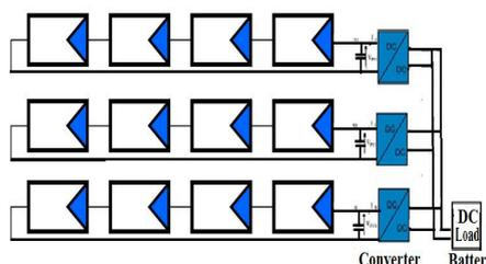
Figure .7: Series connection of a string converter
