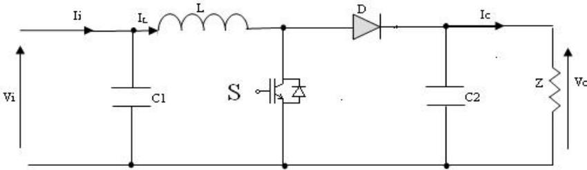
Figure.3: Electrical circuit of boost converter [7]
