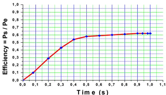
Figure.10. The yield effect in case of single converter damage.
