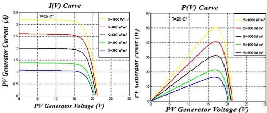
Figure .2: Simulation results for the I(V) and P(V) characteristics of a PV module as a function of different irradiances at T=25°C.
