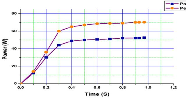
Figure .16 : Power of the string converter connected in series.
